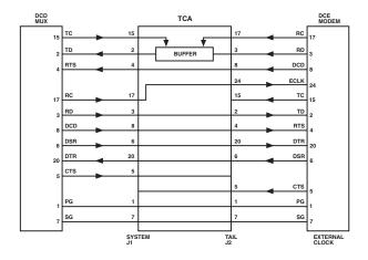
Figure 4-2. Schematic Diagram of Data Flow.
