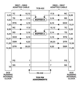
Figure 2. Data Flow Schematic Diagram.
