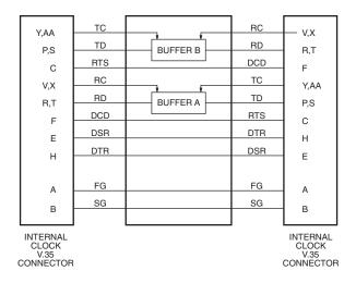
Figure 1. TCB-V.35 schematic.
