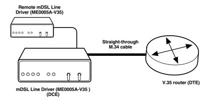
Figure 4-2. Connecting the Line Driver to a V.35 serial DTE.
