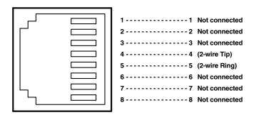
Figure 4-1. RJ-45 twisted-pair line interface.
