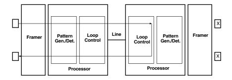
Figure 5-7. Block diagram remote loop.
