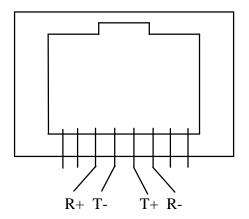
Figure 3: Female RJ-11 and RJ-45 wire designations.
