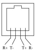
Female RJ-11 mounted on PCB
