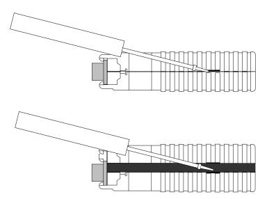
Figure 3-3. Using a screwdriver to open the case.
