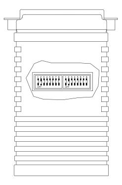
Figure 3-1. The A/SLD's internal configuration switches.
