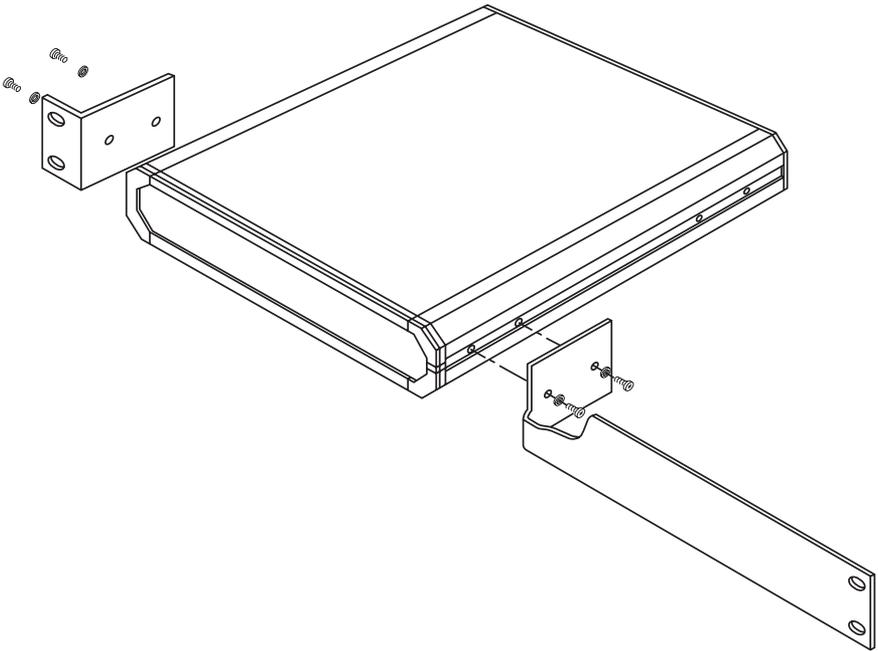
**Figure 4-1. Preparing a single LHM-19.2 for mounting in a 19" rack.**
