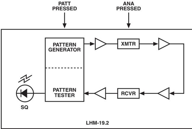
Figure 6-1. Single-modem BERT during local analog loopback.
