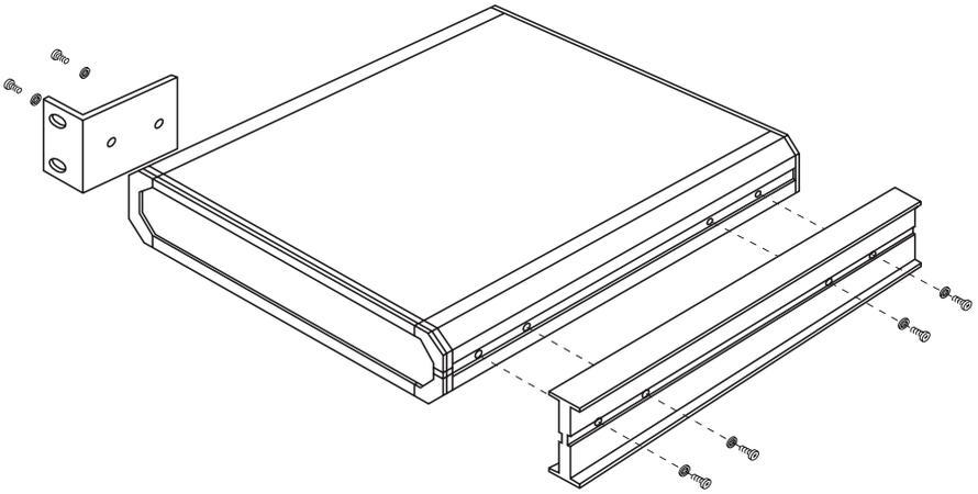
Figure 4-2. Preparing each LHM-19.2 for dual rackmounting.
