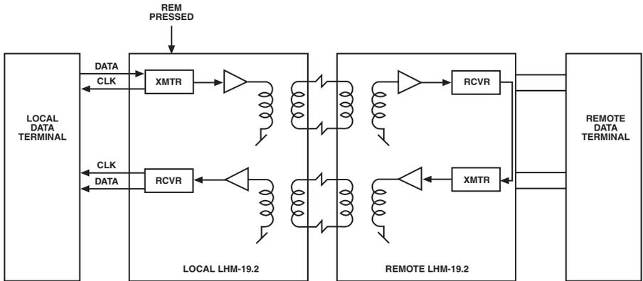
**Figure 6-4. Remote digital loopback.**
