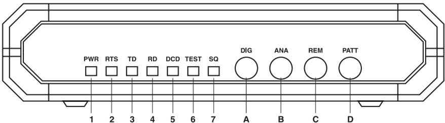
**Figure 5-1.** The LHM-19.2's front panel.
