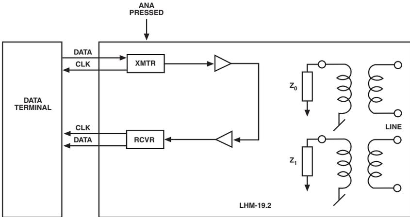
Figure 6-3. Local analog loopback.
