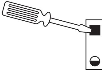
3. Insert the stripped end of the wire and remove the screwdriver. The clamp will close and the wire will be securely connected.
