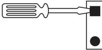
2. Lever the screwdriver handle upwards to put pressure on the element at the bottom of the square hole. The terminal's wire clamp will open.
