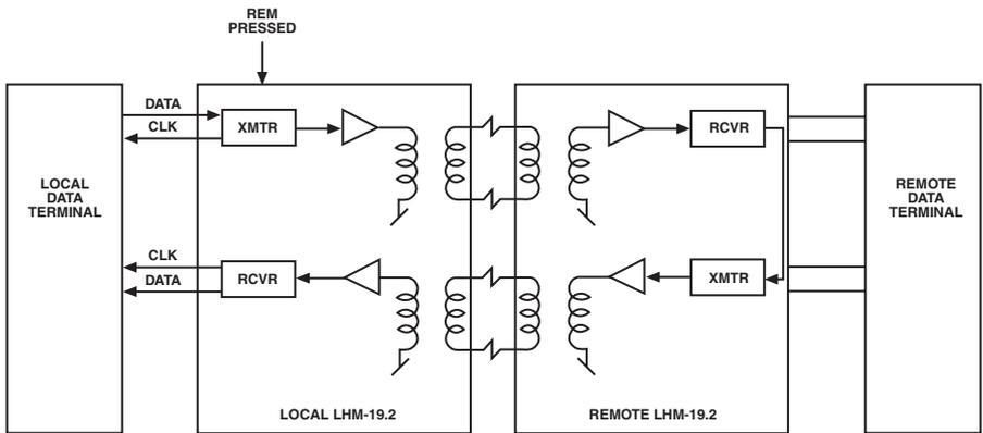
**Figure 6-4. Remote digital loopback.**
