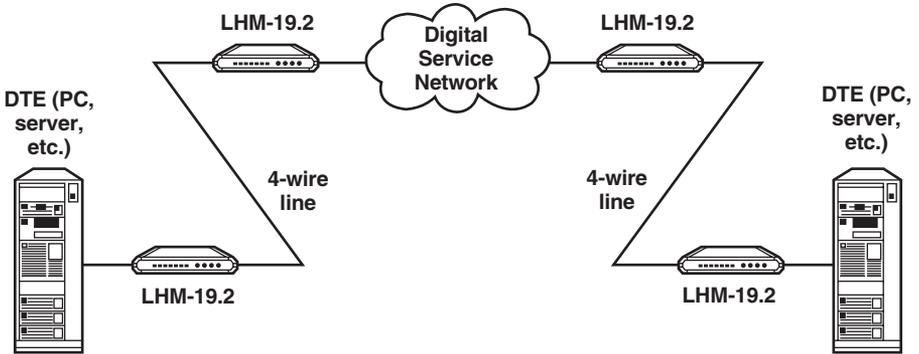
Figure 2-2. Four LHM-19.2s in a tail-circuit application.
