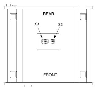
Figure 3-1. External DIP-Switch Locations.
