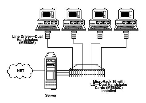
Figure 1. Install a MicroRack-16 chassis in your control room and fill it with LD—Dual Handshake Cards. Then connect your remote user sites to your central hub using plug-in Line Driver—Dual Handshakes (part number ME680A-M, ME680A-F, ME681A-M, ME681A-F, ME680AE-M, ME680AE-F, ME681AE-M, or ME681AE-F) and twisted-pair wiring. Now your multiport host or terminal server can become a cost-saving Internet server.
