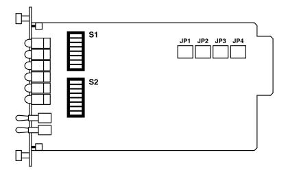
Figure 2. Location of the DIP switches.
