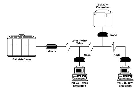
Figure 2-2. Multipoint Synchronous Application.
