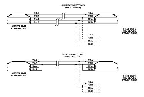
Figure 3-1. Inter-Connect Wiring Diagram.
