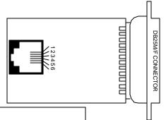
If there is a shield around the telephone cable, it may be connected to "G" on the terminal block. We recommend connecting the shield at the computer end only to avoid ground loops. A ground wire is not necessary to properly operate the Driver.
