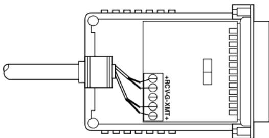
11. Bend the top half of the case to place it over the strain relief assembly. Do not snap the case together.
