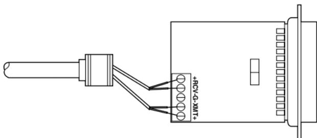
10. Insert the strain-relief assembly, with the wire going through it, into the slot in the bottom half of the modem case and seat it into the recess in the case.
