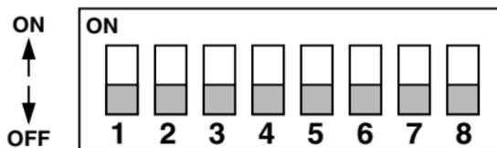
Figure 3-3. Closeup of the DIP switch. All eight switches are ON.
