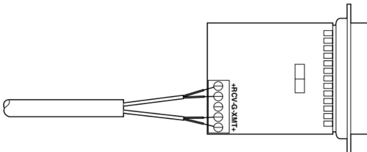
9. Place the two halves of the strain-relief assembly on either side of the telephone wires and press together very lightly. Slide the assembly so that it is about two inches (5 cm) from the terminal posts and press together firmly.
