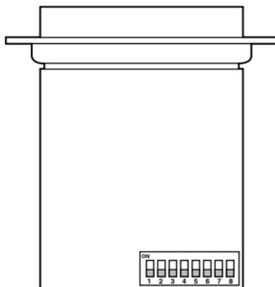
Figure 3-2. Bottom view of the PC board, showing the internal DIP switch.
