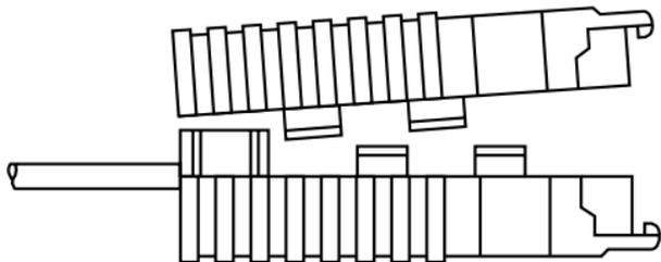
12. Insert one captive screw through a saddle washer and then insert the captive screw with the washer on it, through the hole in the DB25 end of the case. Snap that side of the case closed. Repeat the process for the other side.
