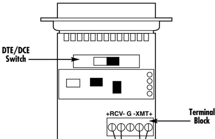
Figure 3-1. The Mini Driver MP board and DTE/DCE switch.
