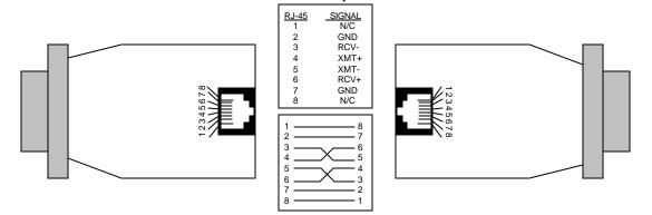
If there is a shield around the telephone cable, it may be connected to "G" (GND)on the RJ-45 connector. To avoid ground loops, we recommend connecting the shield at the computer end only. A ground wire is not necessary for proper operation of the Mini Driver MP9.
