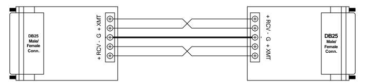
If there is a shield around the telephone cable, it may be connected to "G" on the terminal block. To avoid ground loops, we recommend connecting the shield at the computer end only. A ground wire is not necessary for proper operation of these units.
