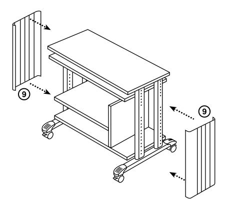
Figure 6. Replacing the plastic cable management slide covers.
