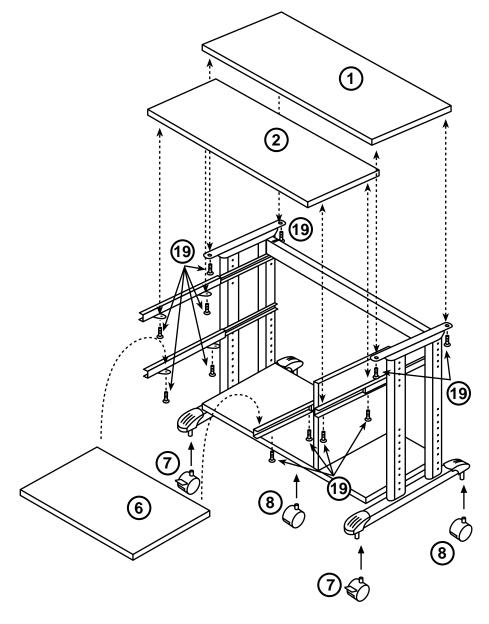
Figure 5. Attaching the casters to the frame.
