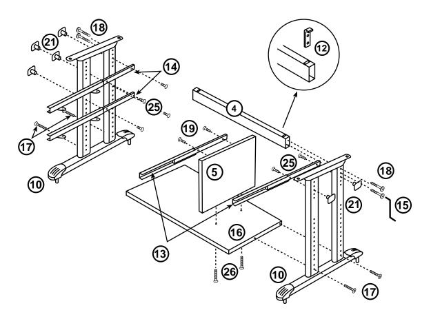
Figure 4. Attaching the monitor surface to the top of the leg assembly.
