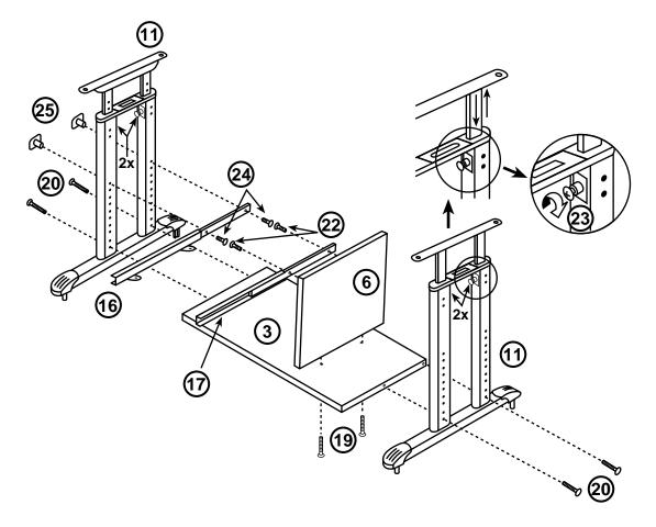
Figure 5. Attaching the monitor surface to the top of the leg assembly.
