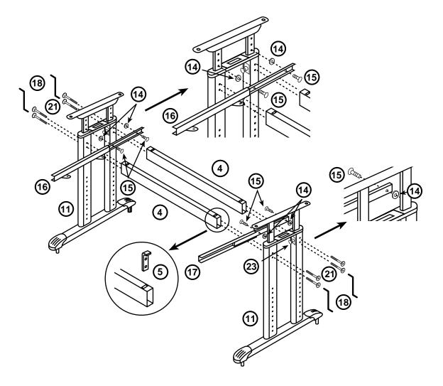
Figure 6. Installing the front and rear steel support cross bars.
