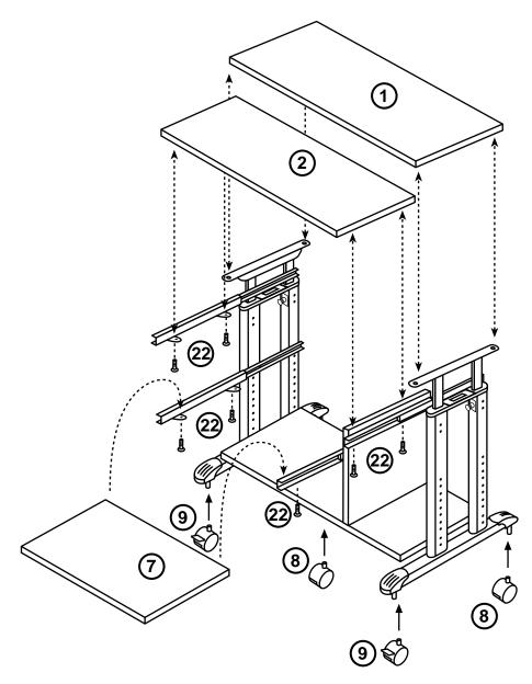
Figure 7. Attaching the casters to the frame.
