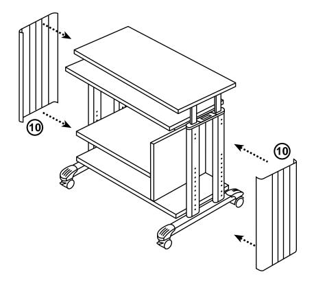
Figure 8. Replacing the plastic cable management slide covers.
