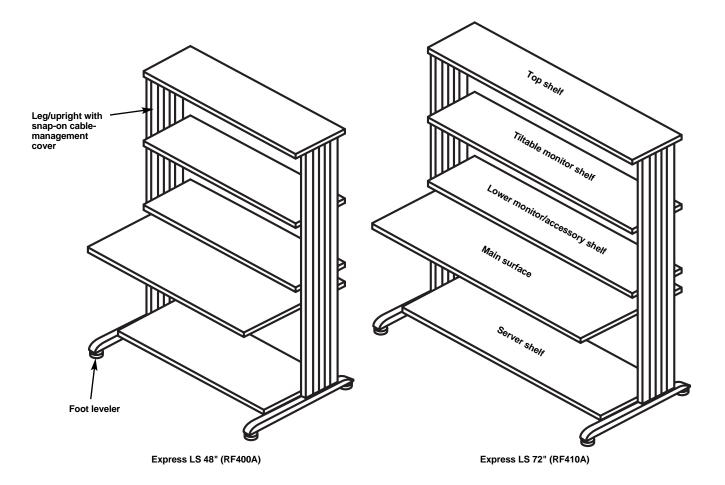
If you ordered the Wire Keyboard Shelf (RF411), you can install it after the Express LS is completely assembled. There are pre-drilled holes for attaching the Shelf to the Express LS; these are located on the under side of the tiltable monitor shelf (see the illustration below). The Wire Keyboard Shelf comes with all of the hardware necessary to attach it.
