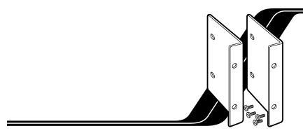
You can use these Rackmount Kits (which consist of two rackmounting "ears" and four screws) to mount a ServSwitch<sup>TM</sup> Affinity in a standard equipment rack:
