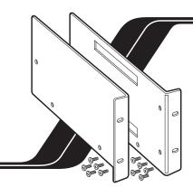
Use a ServSwitch Multi™ Rackmount Kit (our product code RMK19J) to mount a ServSwitch Multi (our product code KV150A or KV160A) in a 19" rack. Each of these Kits consists of two rackmounting side brackets and ten screws. To use a Kit to mount a ServSwitch Multi, take these steps, referring to the illustration below:
