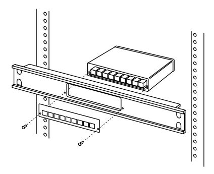
Figure 1. Rackmounting the Hub front forward.
