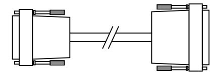
Figure 4-4. DB25 male to DB34 male adapter 6-ft. (1.8-m) cable used to connect the BERT Tester's DB25 pin female interface port (RS-530) to the DCE's DB34 female interface port (V.35).
