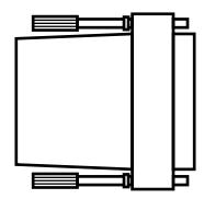
Figure 4-3. DB25 hood used to connect modular cable from the BERT Tester console port to a modem.
