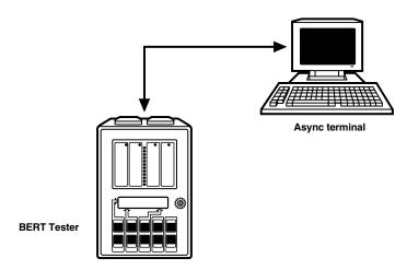
Figure 3-1. Using the BERT Tester to test an async terminal.
