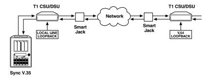
Figure 3-3. Testing a T1 facility with CSU/DSUs and V.35 interfaces.
