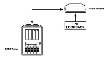
Figure 3-2. Using the BERT Tester to test an async modem.
