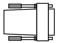
Figure 4-2. DB9 hood used to connect modular cables from the BERT Tester console port to a terminal.
