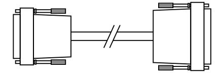
Figure 4-5. DB25 male to DB37 male adapter 6-ft. (1.8-m) cable used to connect the BERT Tester's DB25 female interface port (RS-530) to the DCE's DB37 female interface port (RS-422).
