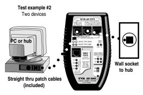
Using 2 leftmost sockets simulates a straight thru connection
