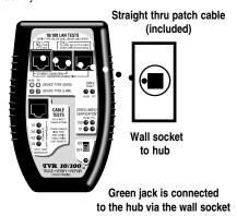
**Step 1:** Connect the hub outlet (at the remote site) to the TVR10/100's Main Unit GREEN JACK (use the straight thru RJ45 patch cable that is provided).
