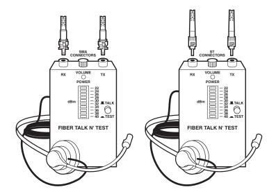
Fig. 2-2. The Fiber Talk N' Test.
