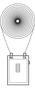
Fig. 3-1. Measuring the Loss in a Spool of Fiberoptic Cable.
