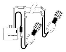
2. With the test set in the CONT position, a "dead line" is supplied with talk power.
