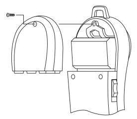
Figure 3-2. Replacing the battery.
