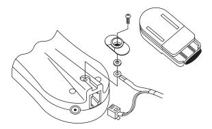
Figure 3-3. Attaching the belt clip.
