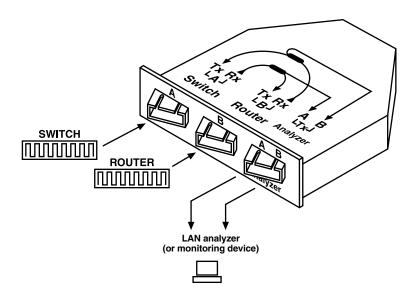
Figure 2. Attaching devices to the splitter module (internal data flow also shown).
