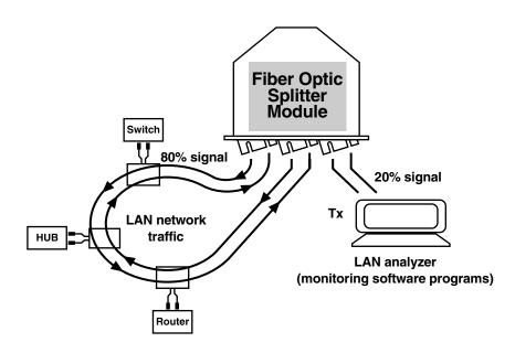
Figure 3. Total data flow when used in a ring network.
