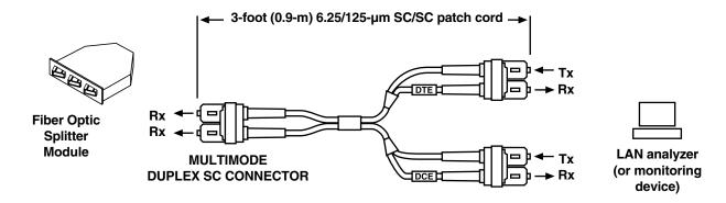
Figure 1. The Fiber Optic Analyzer Patch Cable (EFN4029-CT).
