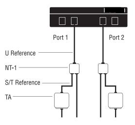
Figure 3 S/T Interface operation
