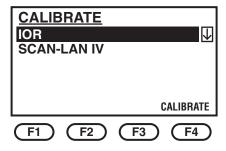
You can use system-default IOR settings, manually input new settings, or calculate the correct IOR based on a known length of cable.
