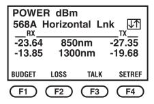
To establish a new reference after initially setting the reference, return to the Power screen by pressing ESC while the Loss screen is shown.
