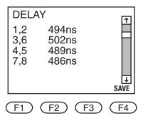
Press the down arrow to view Delay Skew test summary. This screen shows the additional delay time for each pair, compared to the shortest pair.
