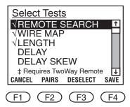
5. Press PAIRS (F2) to select which wire pairs will be included in the tests (twisted-pair cables).
