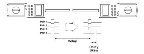
Delay and Delay Skew are tested only during an Autotest or Quick Check. They are included in Autotest for the enhanced cable standards (for example, CAT5 Plus BasicLink). These tests can be added to Autotest or Quick Check for any other cable standard by defining a custom cable standard (see **Appendix A**).
