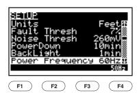
• Press 60Hz/50Hz (F4) to change the power-frequency setting.
