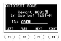
After saving, a message in the upper right corner of the screen displays the saved report number (for example, "Saved #001").
