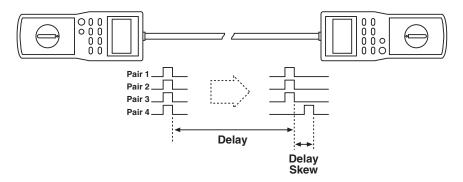
Delay is a measure of the time electrical signals take to propagate from one end of the cable to the other end. The difference in propagation delays from one cable pair to another is called Delay Skew.
