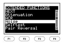
3. Press ENTER to select the test. The test begins immediately. (Press the arrow keys to change the cable test standard.)
