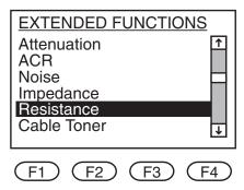
4. Press ENTER to select the test. The test begins immediately. Press ESC to abort the test. (Press the arrow keys to change the cable test standard).
