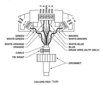
Figure D-3. UTP Cable Assembly.
