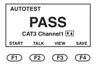
3. When the remote unit enters TALK mode, an alert bell will ring. Press STOP RING (F3) or any other defined function button on the remote unit to stop the bell.
