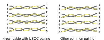
Figure 8-5. Common Wiring Configurations.
