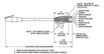
Figure D-2. Cable Preparation per EIA/TIA T568B.
