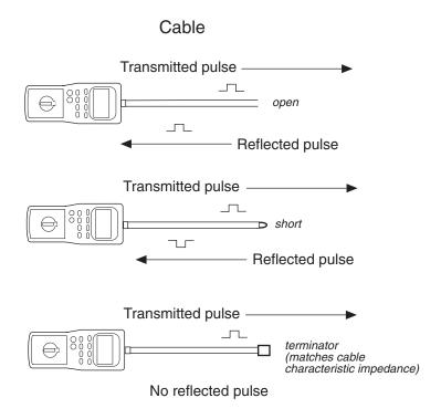
Figure 8-10. Using TDR to Locate Cable Faults.
