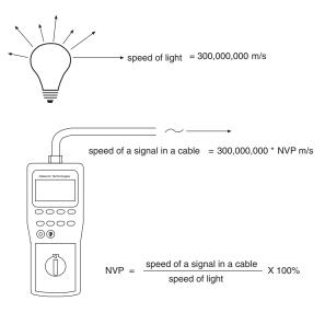
Figure 8-11. Cable Nominal Velocity of Propagation.
