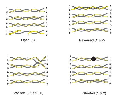
Figure 8-3. Continuity Wiring Errors.
