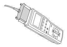
Removing or installing the performance module.
