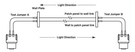
TIA OFSTP-14A measures the installed fiber attenuation plus the loss of the Test Jumper. This is the specified method for testing the multimode cable under TIA/EIA-568A and ISO/JEC 11801, and is appropriate when measuring a cable plant with patch panels on both ends, or with a patch panel at one end and a wall outlet at the other.
