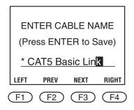
9. Press ENTER to save the custom cable test standard.
