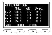
2. Press SEND (F1) to restart the Attenuation test.
