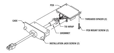
Figure D-1. Performance Module Disassembly.
