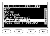
4. Press ENTER. Press ESC to abort the test. (Press the arrow keys to select another cable test standard.)
