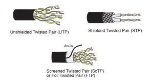
Figure 8-1. Twisted-Pair Cable Construction.
