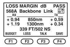
The Margin screen displays the amount of headroom between the allowable loss in the selected cable standard and the measured loss in the cables under test.
