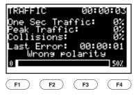
Figure 11-2. Traffic Test Results Screen (No Link Pulse).
