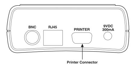
Fig. 6-1. Printer Connector on the Scanner.
