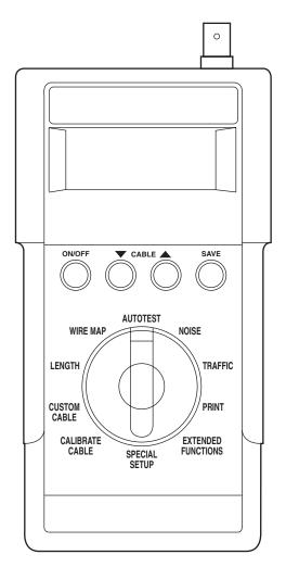
Fig. 2-2. SCAN-LAN 150 Cable Scanner.
