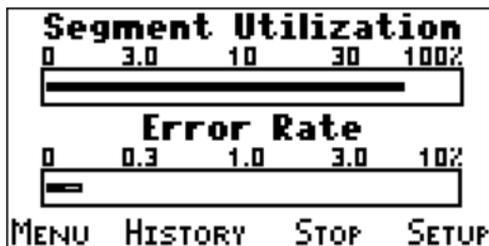
2. Press **STOP (F3)** at any time to stop LAN Monitor data collection. To restart LAN Monitor data collection, press **START (F3)**. The LAN Monitor will begin collecting new data (previously collected data will be discarded).
