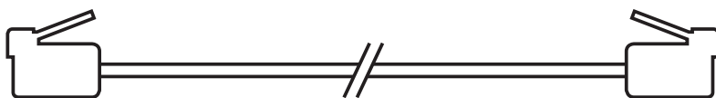
Figure 4-1. RJ-11C 6-pin modular to modular straight-through 6-ft. (1.8-m) cable—WAN Tester console to DB9 hood when connecting to console.
