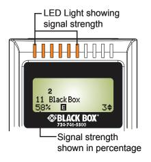
WLANs detected during scan are ordered by channel number and network name (SSID). Use the arrow keys to scroll up and down the list of detected WLANs. The WLANs relative position within the list is depicted by illuminating one of the fixed numbers (1-8) in the numeric sequence above the SSID.
