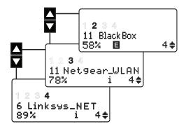
During scanning a ping is sent to the Internet IP every 15 seconds. If a response is received, an Internet indicator (i) is displayed.
